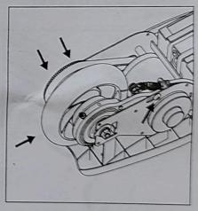
Install replacement wheel into the frame and slide belt back onto the pulley. Do not tighten axle nuts yet. Install brake arm hardware, do not tighten yet.
