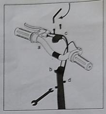
Align handlebars both vertically and horizontally (a) onto handlebar steer tube clamp (b) install handlebar clamp and hardware (c&d) and tighten evenly and securely with the 5mm hex wrench and 10mm wrench.
