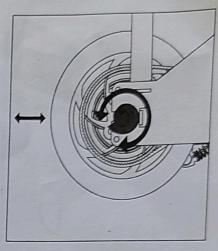
Rotate the adjustment washers against the frame tab to increase or decrease the belt tension. The recommended belt tension is based off of being able to twist the belt approximately 90 degrees.
