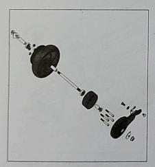
4. Note the location of all rear wheel hardware and ensure to properly reinstall all items.
