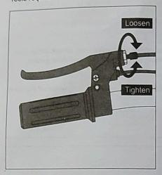
1. To adjust the brake cable thread clockwise (loosen) or counter clockwise (tighten) the adjuster barrel on the brake lever. Only turn the barrel in small increments until the desired adjustment is reached. If brake continues to need further adjustment proceed to the next step.
