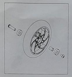
Reinstall new replacement wheel ensuring to note the order and location of all components.
