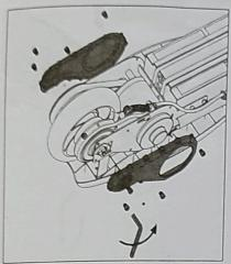
Using a 4mm hex wrench remove the 4 protective cover bolts on both sides of the conter.
