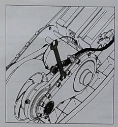
2. If the brake cable is still either too tight or too loose use a 10mm wrench to loosen the brake cable pinch bolt for further adjustment on the cable. Ensure that the 10mm nut is securely tightened after the adjustment is made.
