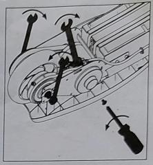
3. Remove the brake arm bolt with a Phillips screwdriver and 8mm wrench. Using two 13mm wrenches loosen the rear wheel axle nuts and adjustment washers and slide the belt off of the rear wheel pulley. Pull the wheel towards the rear of the frame.
