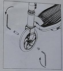
3. Reinstall hardware and tighten clockwise with a 5mm hex wrench.
