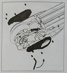
1. Using a 4mm hex wrench remove the 4 bolts from the rear axle cover on both sides of the scooter.
