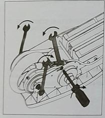
4. Ensure wheel is aligned in the frame and tighten the two axle nuts with a 13mm wrench. Retighten the brake arm bolt with a Phillips screwdriver and 8mm wrench.
