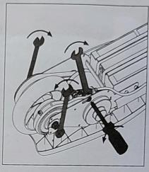
Loosen the brake arm bolt with a Phillips screwdriver & 8 mm wrench. Using two
