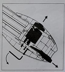
5. If replacing the belt remove the motor bolts with a 5mm hex wrench. Slide motor out of the frame slightly so that there is enough room to remove/replace the belt onto the motor gear. Replace spacers and retighten bolts.
