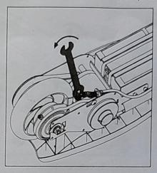
2. Loosen brake cable pinch nut with 10mm wrench.
