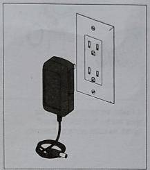
2. Plug the charger into a wall power outlet. The light on the charger housing should illuminate. Red LED light indicates battery is charging and a green LED light indicates battery is fully charged.
