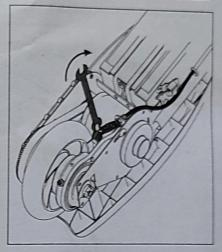
Retighten brake cable pinch nut with 10mm wrench. Refer to the instructions on page 7 for proper adjustment.
