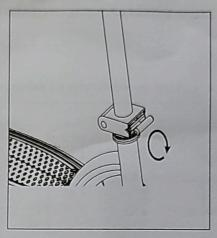
2. Fasten the triangle block on the spiral into the front fork. Twist and tighten the spiral evenly and securely.
