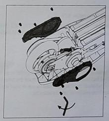
5. Reinstall side covers with a 4mm hex wrench. Do not over tighten bolts.
