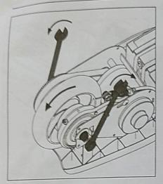
7. Ensure adjustment washers are seated correctly against the frame. After tightening axle nuts with a 13mm wrench check wheel alignment and the tracking of the belt by rotating the wheel counter clockwise with your hand. Adjustment washers may need to be readjusted to align belt. Refer to the instructions on page 10 for proper belt tensioning.
