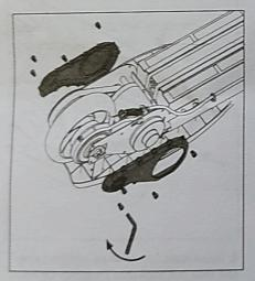
10. Reinstall side covers with a 4mm hex wrench. Do not over tighten bolts.
