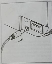
1. Make sure power switch is in the OFF position before plugging in the charger. Insert charger into charging port on the right side of the battery box.
