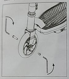
1. Using two 5mm hex wrenches loosen and remove the front axle by turning the wrenches counter clockwise.
