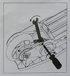
8. Retighten the brake arm bolt with a Phillips screwdriver & 8mm wrench.
