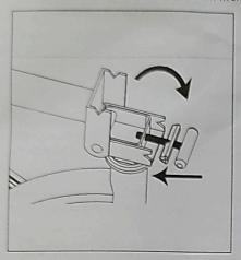
1. As shown in the picture, hold up and align the handlebar steer tube onto the front fork.
