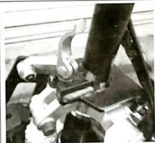
Attach the handlebar by inserting the silver handlebar clamp onto the handlebar post stopping just below the top. Be sure to orient the bars in the correct riding position with the throttle on the rider's right side. Secure the handlebars to the post by tightening the bolts on the clamp with the enclosed Allen wrench as shown.
