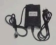
When first plugged in, the charger has one red light that will illuminate at the same time, indicating that the charging process has started. Once the light on the charger turns green, you may remove the charger and close the safety cap.
