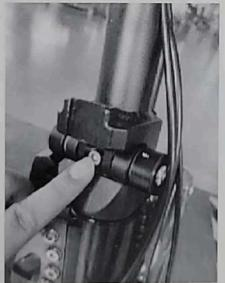
9.when you feel the folding parts too loose or shaking.you can use a wrench to tighten this screw.
